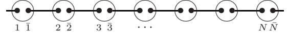
FIG. 1. The schematic of the VBS states with a built-in Lie group G . Each dot denotes a virtual particle transforming under G_D irreducible representations of Lie group G . The solid lines represent valence-bond singlets formed by two virtual G_D irreducible representations on the neighboring sites and the circles denote the projections of the virtual particles in each lattice site onto the physical G_d irreducible representations.
